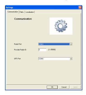
To identify the Ports in your computer in which the Radio and GPS receiver are connected go to Start/Control Panel/System/Hardware/Device Manager/Ports(Com & LPT)
